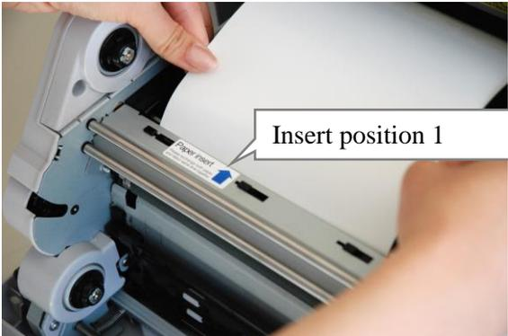
5. Fit the paper to the proper position for each size.
