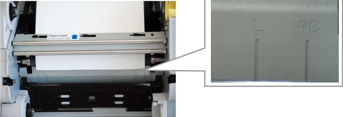
6. Insert the paper under the black paper guide until the buzzer beeps (approx. to the dotted line). Make sure to insert the paper straight. If it isn't inserted straight, the paper will be crooked, which could cause white line on the edges of the print, ribbon wrinkles, and register slippage.
