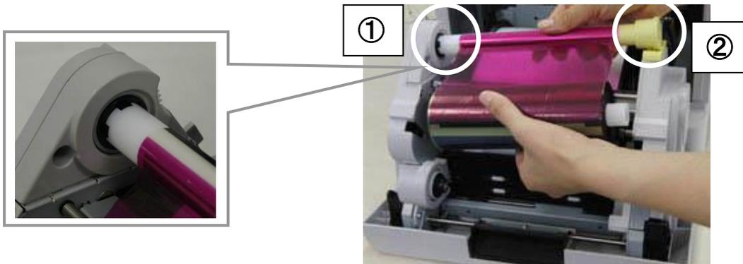
8. Set the supply side of the ribbon to the printer carefully to take out any slack. Insert the protrusion of the core left side in the hole on the printer, then set the right side to the holder of the same color (white). Take up the ribbon slack by rotating the ribbon on the supply side.
