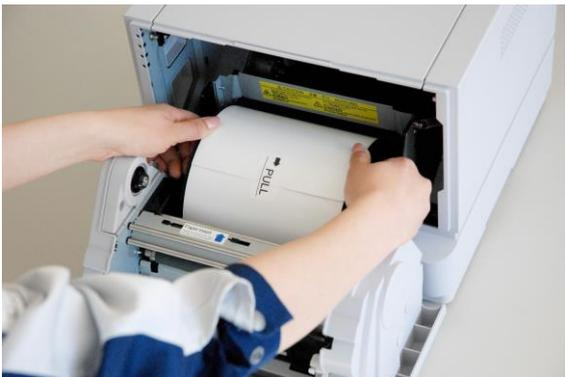
4. Remove a paper fixed tape, and Insert the paper.
