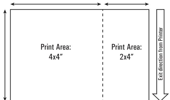
The DS40 printer recognizes media as a standard 4x6 sheet. Layout design is user-defined and needs to accommodate the perforation.
