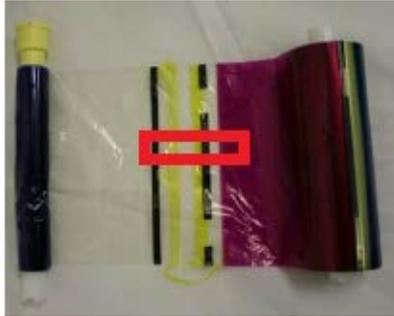
4. Replace the ribbon in the printer and wind the ribbon a few times to remove any slack and until the tape is no longer seen.
