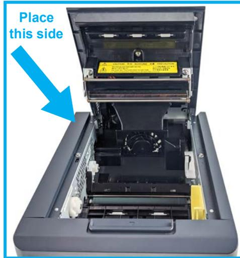
5. Remove any slack from the ribbon by rotating the ribbon towards the supply side.
