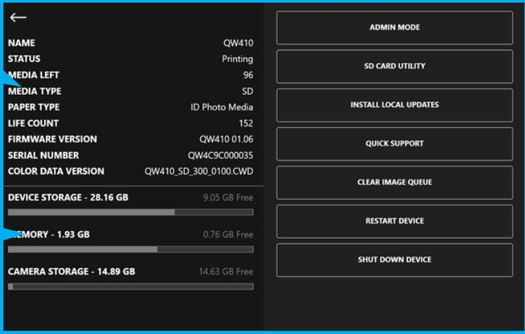
The screenshot displays the printer maintenance screen for a QW410 printer. The left side shows printer information and status, while the right side contains a list of maintenance actions. Blue arrows point from the text labels to the corresponding sections in the screenshot.
