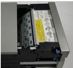
1. Pull any paper remaining in the printer in the direction shown, and cut off any wrinkled or partially printed areas evenly with scissors.
