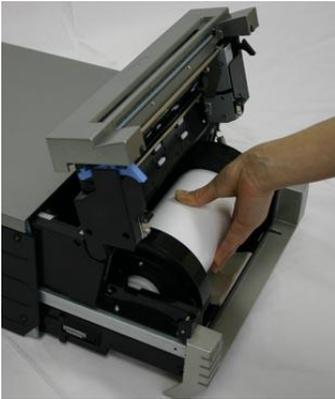
3. Cut off any partially printed, wrinkled, or otherwise inferior paper evenly with a pair of scissors, and reset the paper. If wrinkles or partially printed areas are left, it could cause the paper to jam again.
