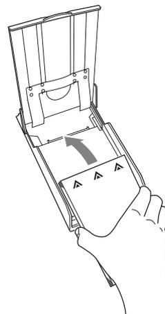
Insert the print paper with the protective sheet facing up and the arrow on the protective sheet pointing in the same direction as the arrow on the tray. You can load 25 sheets when using the UPC-X46 print pack, and 30 sheets when using the UPC-X34 print pack.
