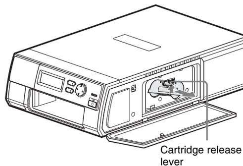
Remove the print cartridge when it ejects.
