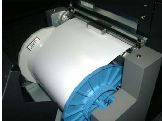
Figure 5. Pinch Roller Label
