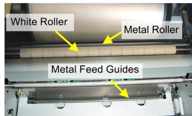
12. Continue sliding the paper through the feed path and between the metal guides until the edge of the paper is visible through the three holes on the metal feed guide.
