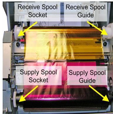
4. Wind the receive spool towards the back of the printer to remove slack from the ribbon.
