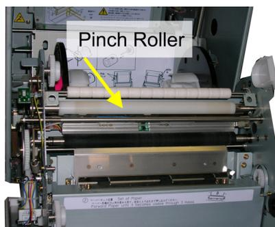
4. Replace the pinch roller guide in the printer by placing the guide in place and securing the black knobs.
