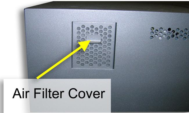
Figure 40. Air Filter Cover Location
