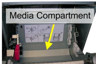
11. Insert the paper between the white and metal rollers and through the paper guides.
