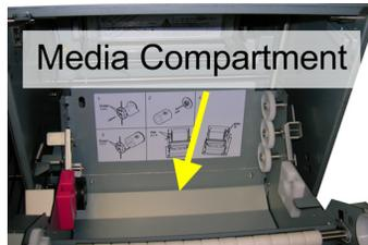
2. Remove the pinch roller guide from the printer by pulling up on the black roller guide knobs and removing the guide.
