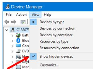
Figure 4.2.2.ii Displaying the View menu for hidden devices
