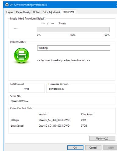
Figure 2.2.6.2 Display when incorrect media is loaded
