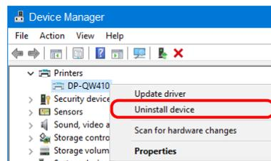
Figure 4.2.2.iii Displaying the menu to delete DP-QW410
