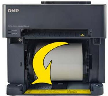
6. **Replace the scrap bin.** Reset the scrap bin in the printer.
