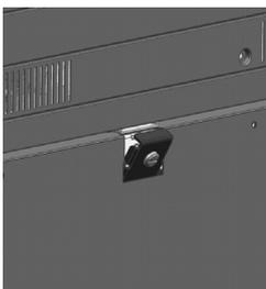
Check that the guide pins on both sides are inserted in the holes at the bottom of the printer.
