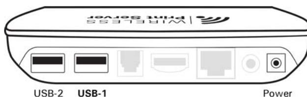
Figure 1. WPS-1 Back View of Ports
