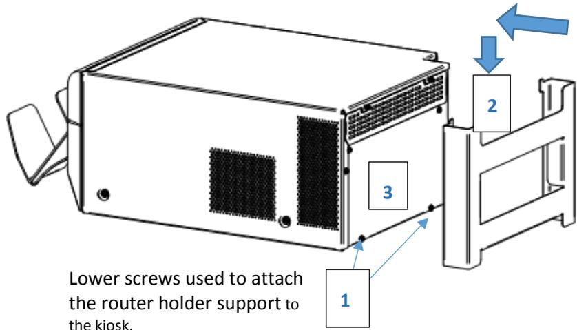
4. Remove the two top screws on DS620A back panel.
