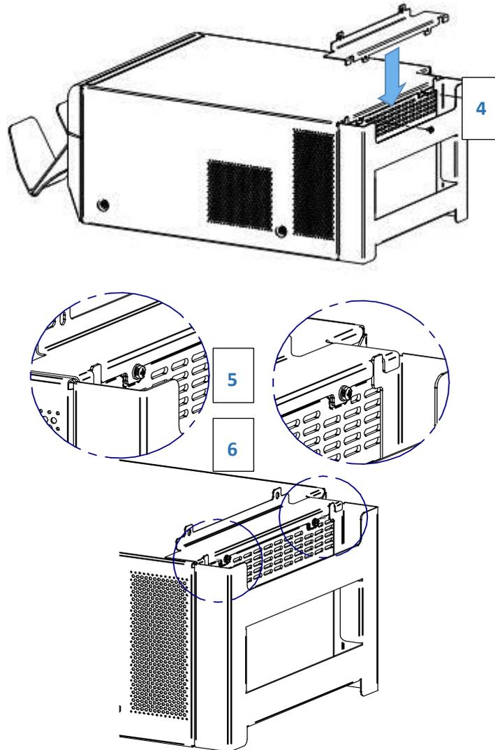
7. Insert the Wi-Fi router into the router support.
